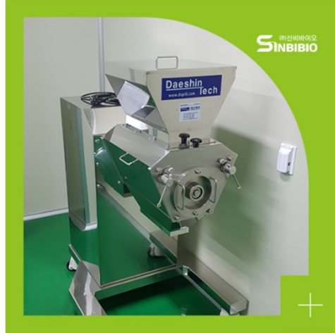
정립기(과립기) (Granulating machine)
